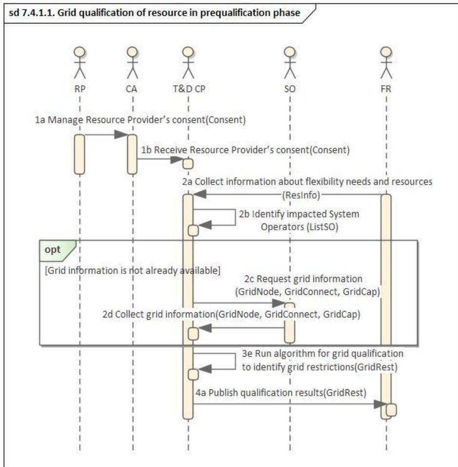
Figure 2.1 Grid qualification of resource in prequalification phase
