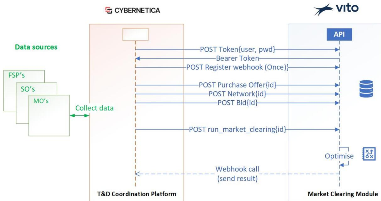
Figure 4.5 API and T&D Coordination platform integration
