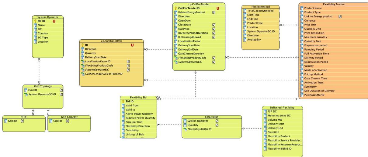
Figure 3.2 Conceptual data model for TSO-DSO Coordination Platform
