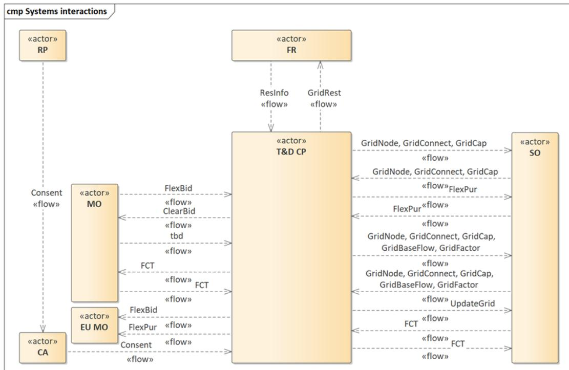
Figure 2.4 Processes of TSO-DSO Coordination Platform within OneNet Northern demonstrator
