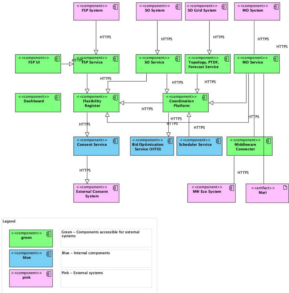
Figure 3.1 T&D CP components
