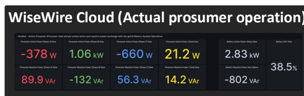
Figure 37: Validation of the precise integration of the actual prosumer in the Cyprus demo digital twin. (a) Monitoring of the distribution grid's digital twin operation through the ABCM-D platform where the actual prosumer is replicated as well, (b) Monitoring of the actual prosumer operation according to the WiseWire cloud interface for the corresponding instant.
