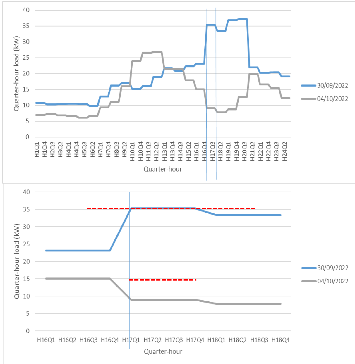
Figure 7-86: FSP-UFD-01 Renewable Energy demonstration center quarter-hour daily load evolution (kW) / Activation time zoomed in
