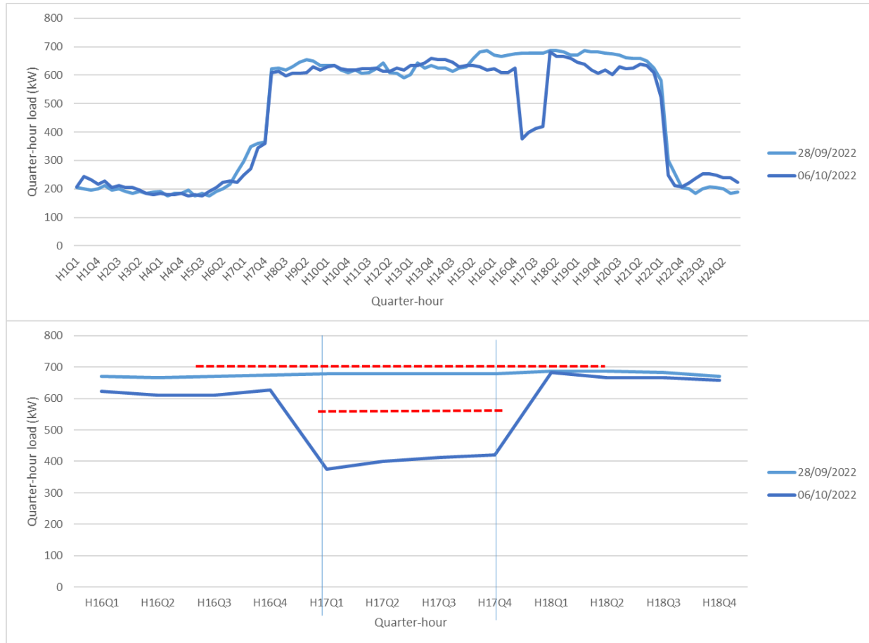
Figure 7-94: FSP-UFD-04 Fiesta Colombina load (kW) quarter-hour daily load evolution (kW) / Activation period zoomed in
