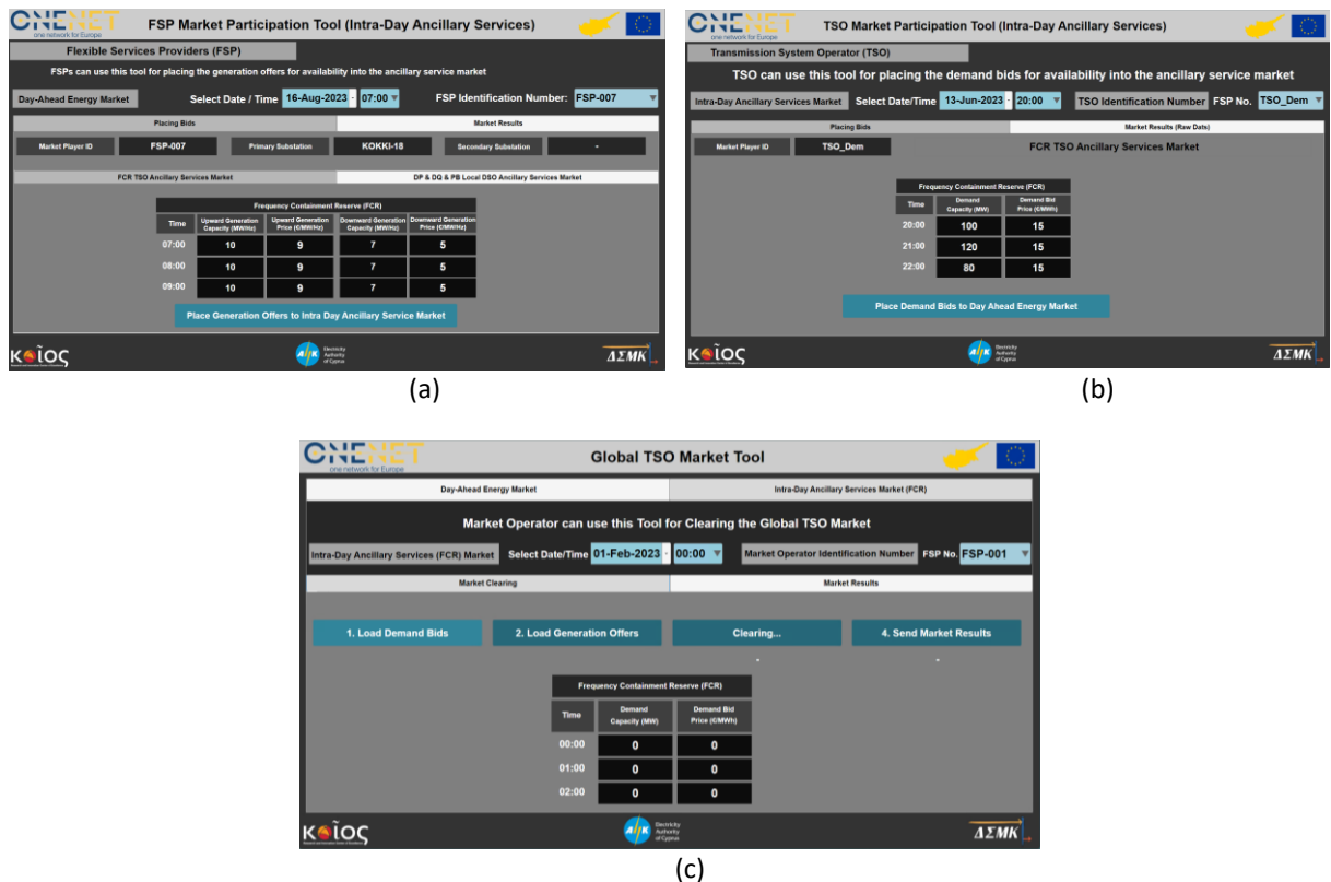
Figure 5: Developed tools for Intra-day TSO FCR Ancillary Services Market: (a) FSP, (b) TSO Market Participation, (c) Global TSO Market Operator
