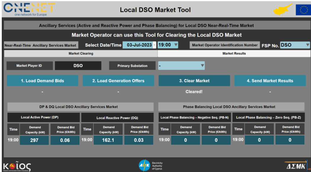
Figure 20: Developed user interface for market operator to clear \Delta P , \Delta Q and PB products and inform all the market participants about the results.
