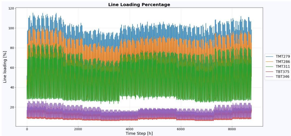
Figure 5.12: Representative yearly line loading profiles for main feeders of Murcian network
