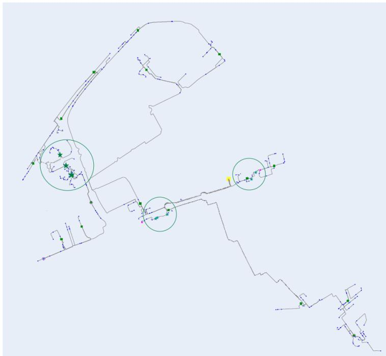
Figure 5.17: Equivalent network for the Alcalá de Henares case study with additional loads location (green-star markers). The green circles highlight the three areas in which the additional load for scenario 1 are connected.
