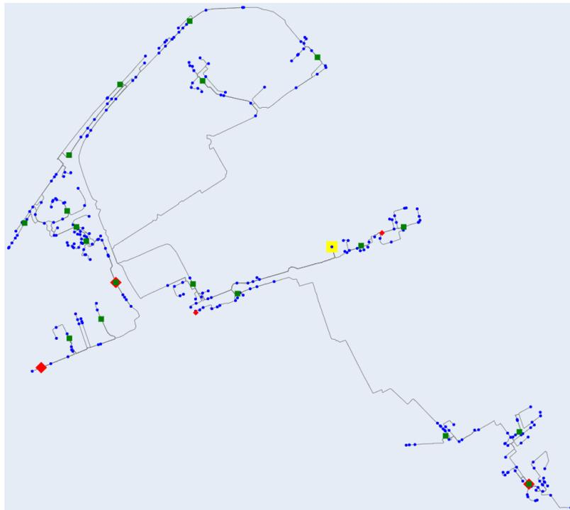
*Figure 5.16: Equivalent network for the Alcalá de Henares case study with SPs location (red-squared markers) and MV/LV transformers location (green-squared markers)*
