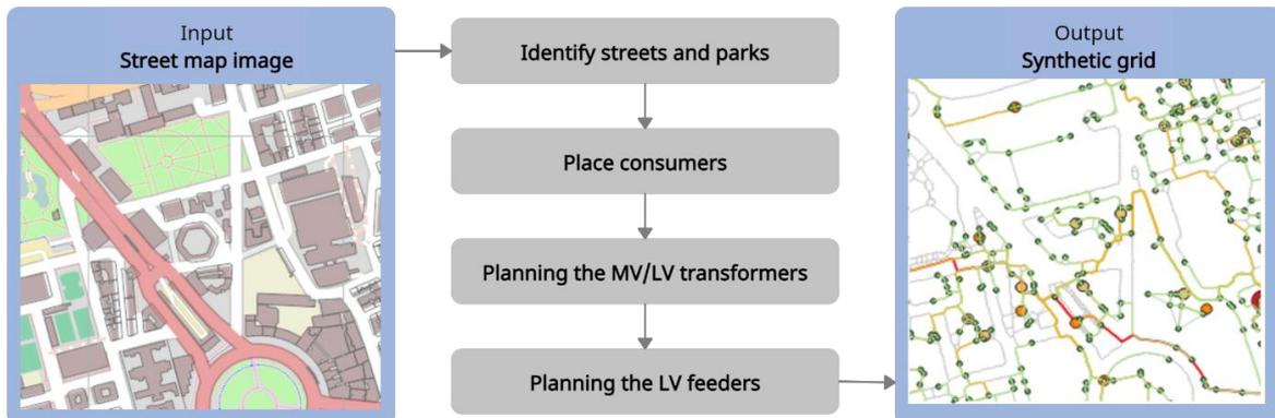
Figure 5.1: RNM approach for designing synthetic distribution grid models [38], [39]
