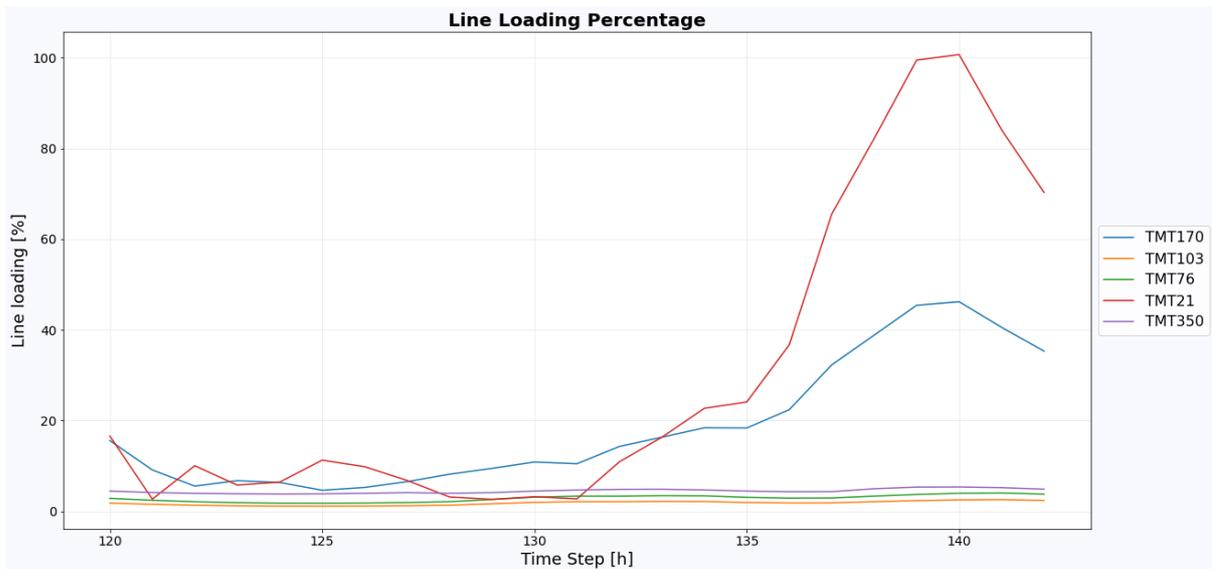
Figure 5.20: Representative day line loading profiles for congestion detection in Alcalá network
