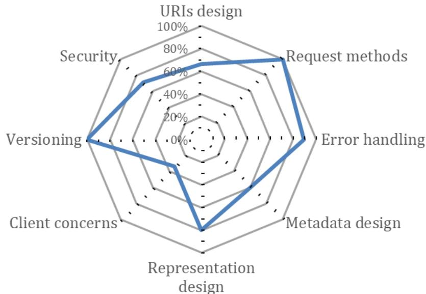
Figure 4.2: Compliance of the French demo API with the best practices for the design of REST APIs that have an impact on its scalability and replicability.
