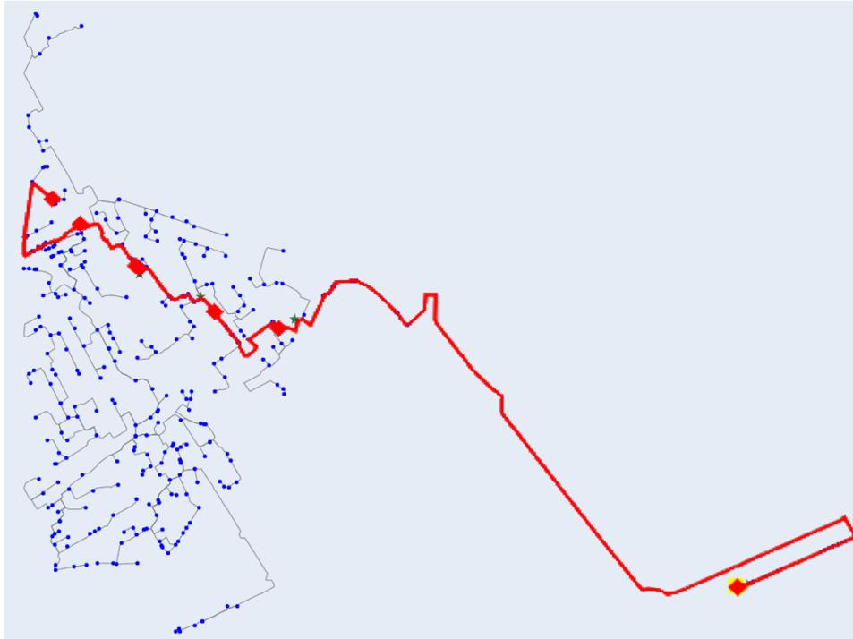
*Figure 5.21: Equivalent network for the Murcian case study with EV charging station location (green-star markers) and the congested elements (red line)*
