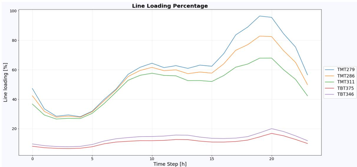
Figure 5.14: Representative day line loading profiles for congestion detection in Murcian network
