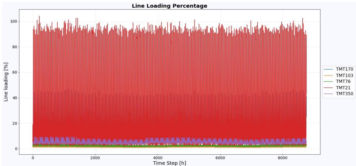
Figure 5.18: Representative yearly line loading profiles for main feeders of Alcalá network
